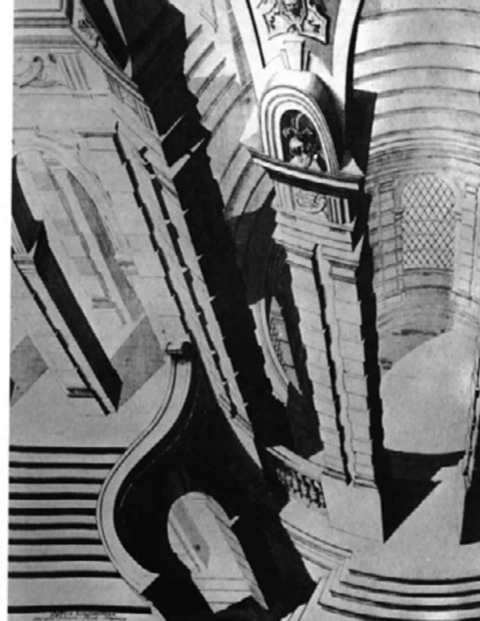
Two examples of "looking down." Note the downward convergence of vertical lines.
