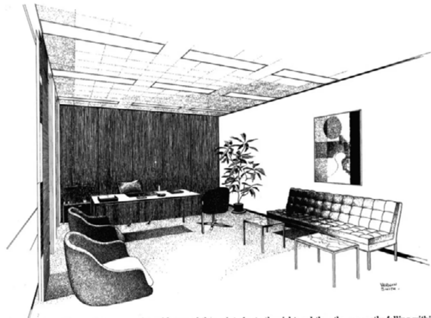
An example of "two-point" perspective with one of the points far to the right and the other correctly falling within the picture. Rendering by Vernon Smith
