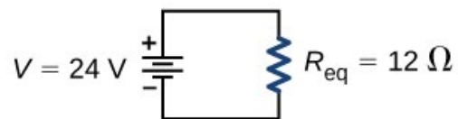
(e) Simplified schematic reflecting equivalent resistance R_{eq}
