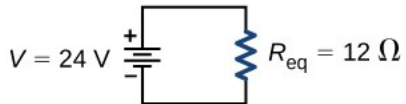
(e) Simplified schematic reflecting equivalent resistance R_{eq}
